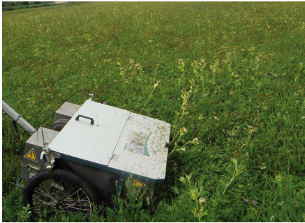
Harvesting with the E-Beetle: Using a brush system, seeds are brushed out of the species-rich meadows.
